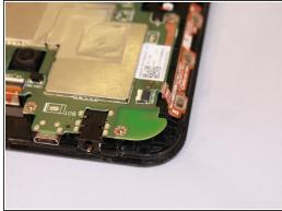
Use the wide nosed tweezers to gently pull out the orange ribbon inserted in the port on the motherboard.
