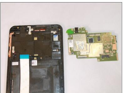
To uninstall the motherboard, use the metal spudger tool to lift it out of the device.
