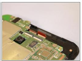
Use the needle nosed tweezers to gently pull both of the orange ribbon cables out of their ports.
