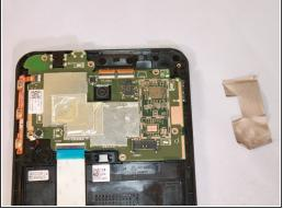
Remove the silver tape on one corner with the needle nosed tweezers, and remove the tape from the motherboard.
