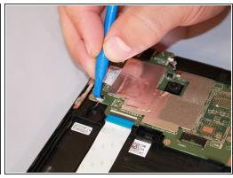
Use a plastic opening tool to slide the white cable connector completely out of the port.
