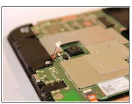
• Use a plastic opening tool to push the white cable connector out of its port in a side to side motion.
