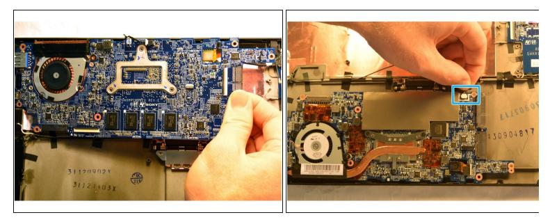
• Gently pull the motherboard out by pulling from the right side of the board and flip it so that the motherboard now sits where the battery was and the underside is now visible.
