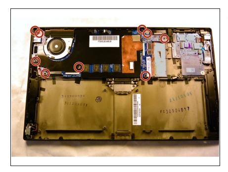
• Remove the nine 3 mm Phillips #000 screws holding in the motherboard.
