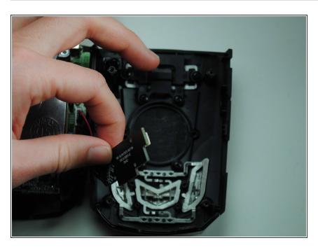
Lift buttonboard to expose silver button plate.
