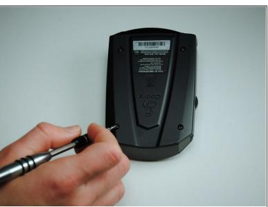
Remove the four 9.5 mm Phillips #0 screws from the back of the device.
