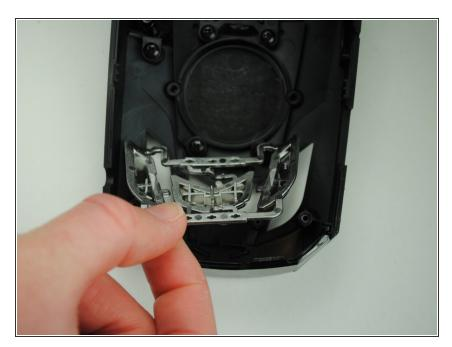
Remove the silver button plate by gripping one of the corners and pulling up.
