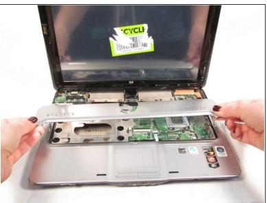
Rotate the screen 90 degrees and remove the base under the screen.
