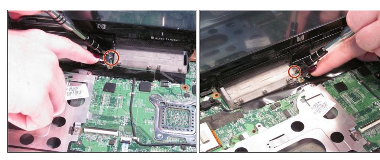
Using the Phillips #0 screwdriver, remove both of the 5.0 mm screws on the base of the rotator.
