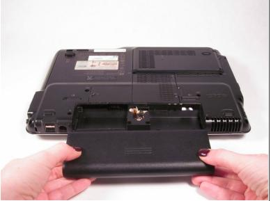
Squeeze the latches on the battery until you hear a click. Slide out the battery.
