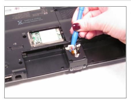
Use the plastic opening tool to disconnect the wires in the upper corners.
