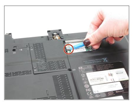
Using the plastic opening tool, disconnect the WLAN antenna cables from the WLAN module.
