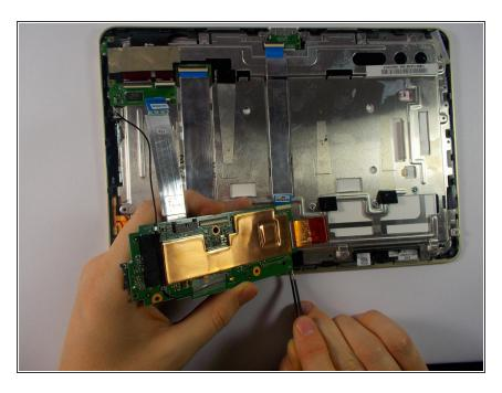
Unhook the camera's ribbon cable from the underside of the motherboard and then remove the motherboard.
