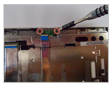
Remove the two keyboard connector screws with the +J000 screwdriver.
