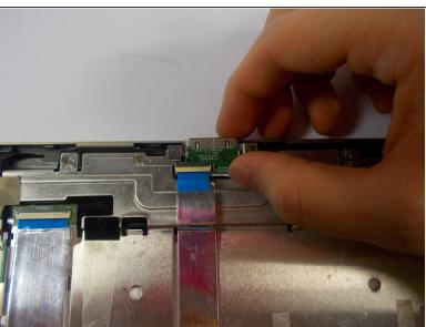
Remove the charging port chip and the keyboard connector chip.
