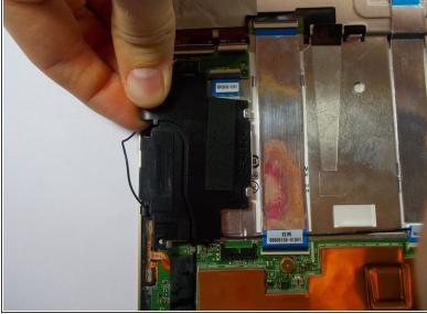
Remove the two speakers from the device's frame
