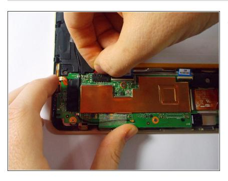
Carefully unplug the battery cable from the motherboard by grabbing the wires close to the black piece and pulling it out of the housing.
