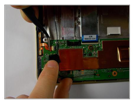
Remove the black tape from the motherboard. Unplug the ribbon cable from the volume and power buttons.
