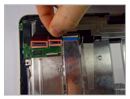
Unplug the two ribbon cables from the charging port chip.
