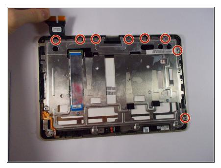
Remove all eight screws from the metal frame with the +J000 screwdriver.
