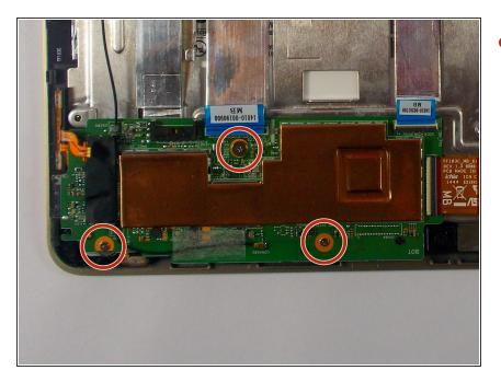
Remove the three screws from the motherboard with the +J000 screwdriver.
