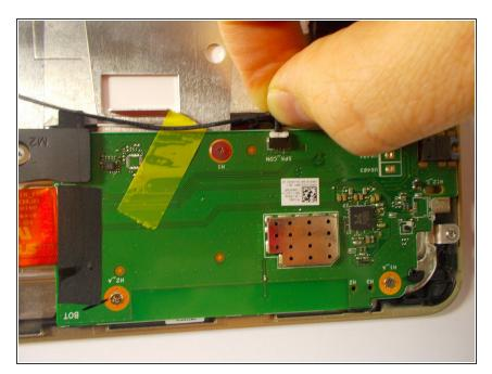
Remove the yellow tape and unplug the wire that attaches the speakers to the soundboard.
