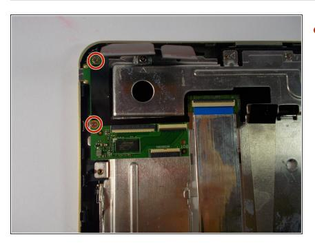
Remove the two charging port screws with the +J000 screwdriver.
