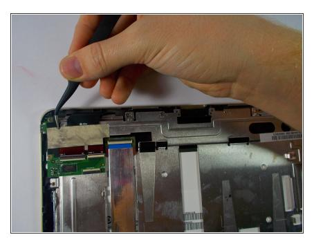
Remove the tape from the charging port chip.
