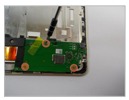
Remove the screws from the soundboard with the +J000 screwdriver.
