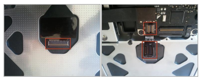
Remove the ribbon cable by releasing it from the ZIF connector on the underside of the trackpad and also from the socket that attaches it to the logic board.
