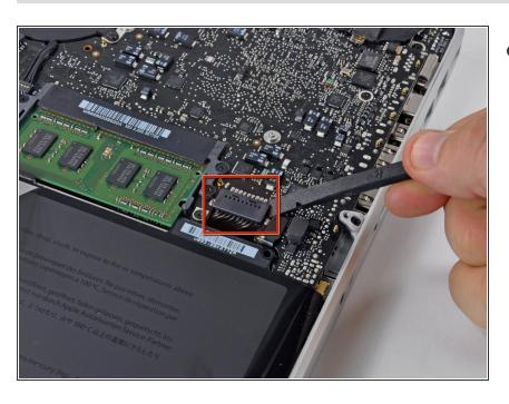
Use the flat end of a spudger to lift the battery connector up out of its socket on the logic board.
