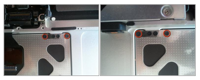
Remove the four 1.2mm #00 Phillips head screws from rear of the trackpad.
