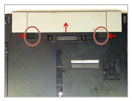
Release the latch or latches connected to the battery that hold it in place.
