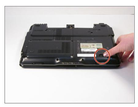
Slide the optical drive release latch on the bottom right side.
