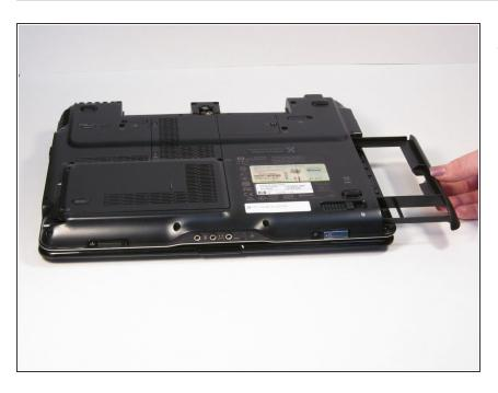
Remove the optical drive from the computer.
