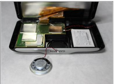
Now using the plastic opening tool, pry the speaker up from one of the sides. Your speaker will completely come out of the device.
