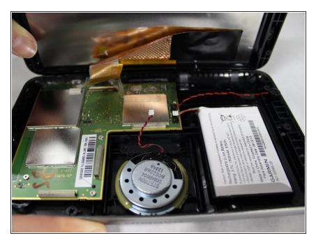
Locate the speaker's wire connector plugged into the motherboard. Now delicately detach the speaker connector by pulling directly up.
