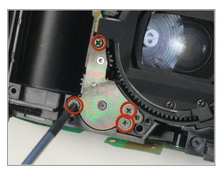
• Unscrew the four screws on the back of this piece to the lower-left corner of the lens.
