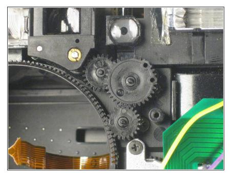
Remove the three gears under the panel you removed in the last step and the lens motor should be able to be removed.
