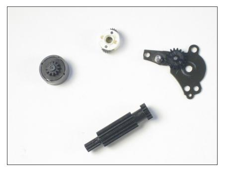
• Removing the lens motor cover, you should be left with these four pieces.
