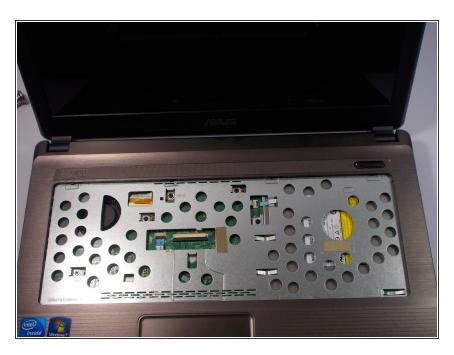
Remove the keyboard completely.
