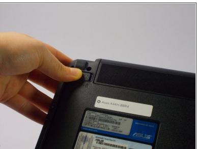
Slide the left lock button into the unlock position and hold.
