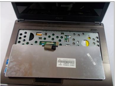
Flip the keyboard over to reveal the back of it and what is underneath.
