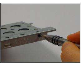
Remove two 3mm Phillips head screws, one located on each side of the metal casing holding the hard drive using the PH0 bit.
