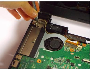
Remove the 5mm Phillips head screw using the PH0 bit.
