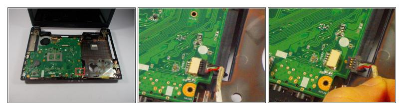
Gently pull out the USB connector attached to the motherboard.
