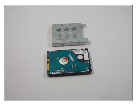
Pull upwards on the metal casing and it will come off.
