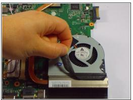
Remove the black piece of tape located on each side of the fan and vent, connecting the two components.
