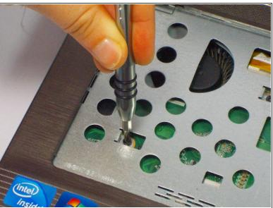
Remove the five 9 mm Phillips head screws with the PH0 bit.
