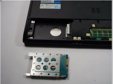
Pull the hard drive upwards and take it out of its position.
