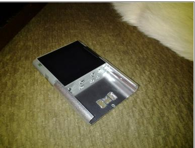
• Basically there is a \*\*TINY\*\* screw just above the belt clip, which must come out (where that very small hole is at the top of the case, centre). I actually used a flat-head watch screwdriver tilted because I didn't have a phillips screwdriver which is what you should use.
