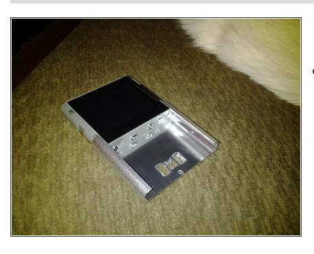
Once I had the screw out it is a simple matter of pushing down vertically on the top portion of the player where all the buttons are - the metal casing will slide down and off. I actually took the belt clip off before I realized it didn't have screws hidden beneath it and I probably could have slid the case off without removing the clip.
