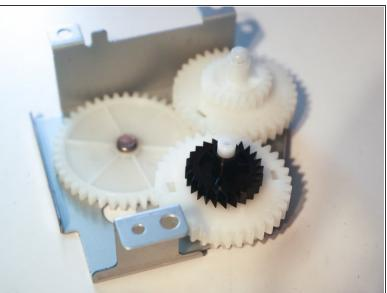
Remove 3 screws holding the duplexer gears to the printer and remove the gears.
