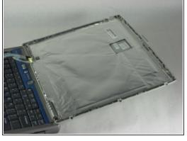
• Remove the cable at the base of the laptop by pulling up on the yellow tab attached to the cable.
