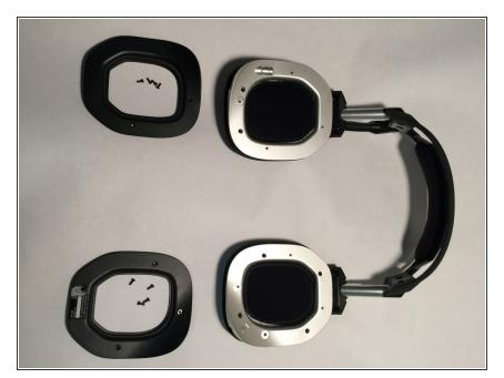
After the screws are removed the black piece of the cover can now come off. Remove this piece.
