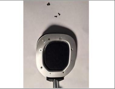
• Then you will see more screws around the now silver edge and a black cushioning pad in the middle. The number of screws depends on the speaker you are replacing, one side has 2 screws while the other has 4.
