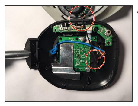
After that take off the cover. If the speaker is still connected and no wires are visibly damaged, then the speaker(s) is not the problem with your device. Please refer back to the troubleshooting page and make sure that the Astro A50 has the newest firmware, etc. If the wire is not connected continue to the next step.
