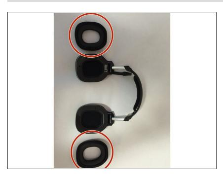
Carefully remove the ear pad from the speaker that the microphone is attached to. Repeat on the other side.
