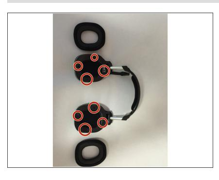
Remove the four screws from each side of the headset.
