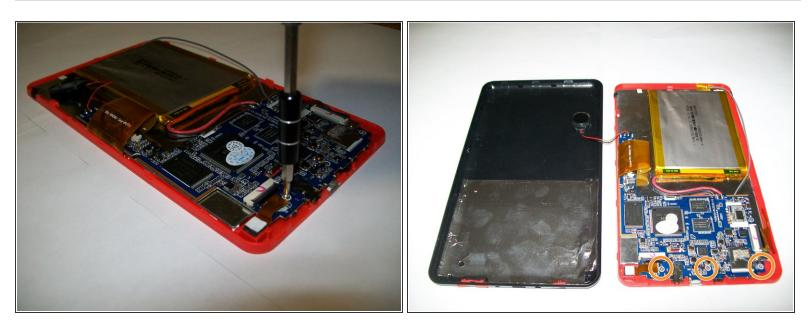
Remove the three screws from the bottom of the motherboard.
