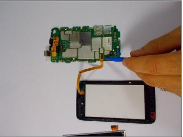
A Remove the ribbon cable connecting the LCD display to the motherboard, be mindful that the ribbon cable is very thin.
