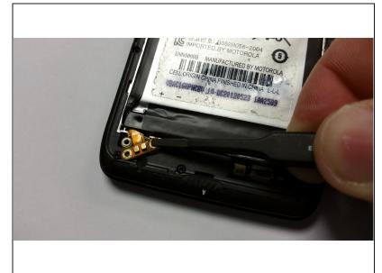
⚠ Lift the battery leads to the upward position. The ribbon cable is very thin, be gentle.
