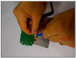
Remove the ribbon cable from the back of the lcd using the plastic opening tool or spudger.
