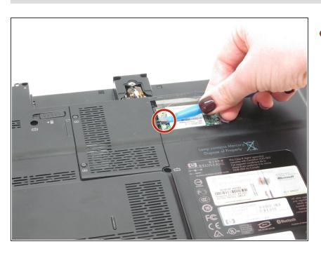
Using the plastic opening tool, disconnect the WLAN antenna cables from the WLAN module.
