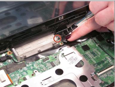
• Using the Phillips #0 screwdriver, remove both of the 5.0 mm screws on the base of the rotator.
