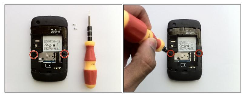
• Remove the two Torx T6 screws to the left and right of the battery.
