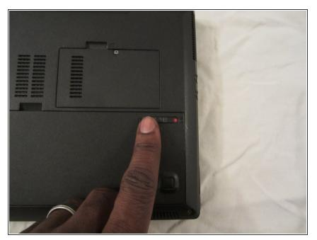
• Locate the sliding tab on the right and slide it to the left in order to unlock the battery.
