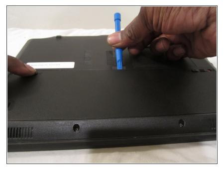
• Use a plastic opening tool to lift the battery up as you slide the tab on the left to the right.
