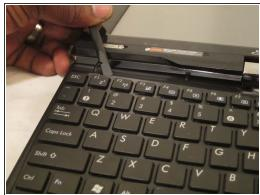
Turn the tablet over and open it up. Insert a nylon spudger into the slots above F1, F6, F10 to pry
