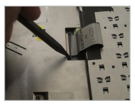
Once you have the keyboard out, use the nylon spudger to remove the connection. You can now replace the keyboard.
