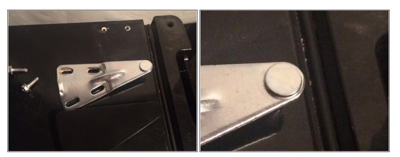
Remove the damaged hinge. Make sure that you don't lose the bolt that goes into the door.
