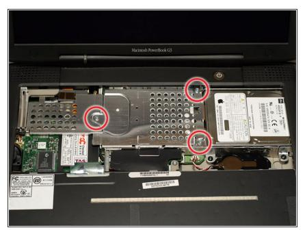
• Remove the three silver Phillips screws that attach the heat shield to the internal metal framework.
