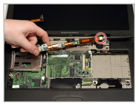
Disconnect the white inverter cable connector from the right end of the board.
