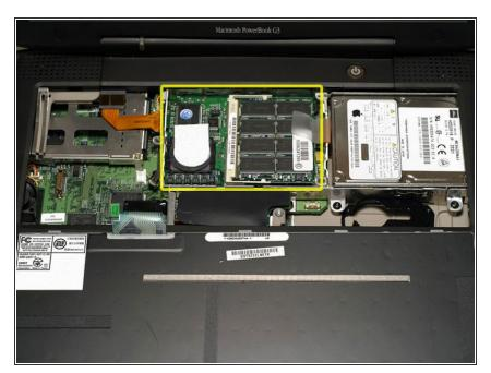
• Use a spudger, the tips of your fingers, or a flat non-metal tool to pry up the processor's right side.
