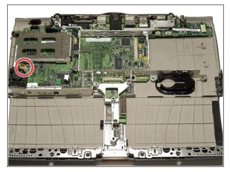
• Disconnect the fan cable from the left side of the logic board.
