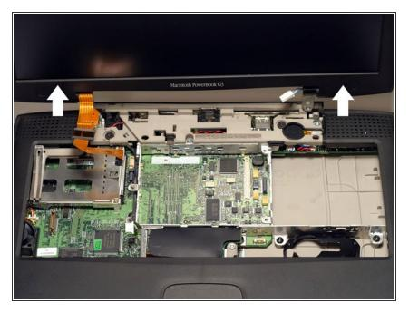
Hold the display on both sides and pull directly up until its hinges are free of their mounts.
