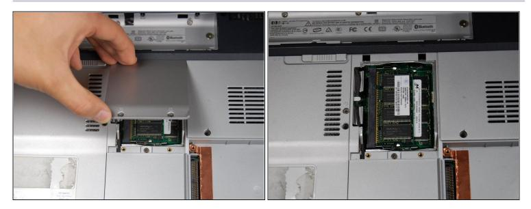
• Lift up on the screw side of the RAM access cover to remove it.
