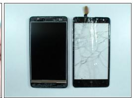
With a cutter separate the glass a little bit to make a room for the plastic pick or other plastic tool.
