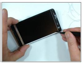
Clean the frame of the old adhesive tape and install new.
