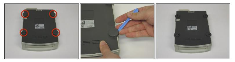
• Pry all four of the plastic feet off the bottom of the enclosure using the iPod opening tool.
