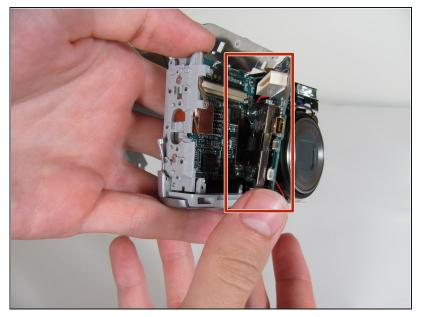
• Remove the motherboard by pulling it up and out of the port.
