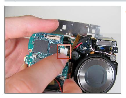
Carefully remove the tab that connects the flash to the motherboard from the port by gently pulling the connector to the right and out of its port.
