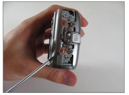
Remove the two 4.8 mm screws attaching the back panel to the body on the left side.
