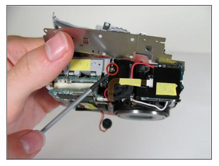
• Remove the 2.8 mm screw from the top of the camera.
