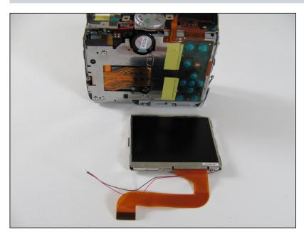
• Remove the LCD from the camera body.
