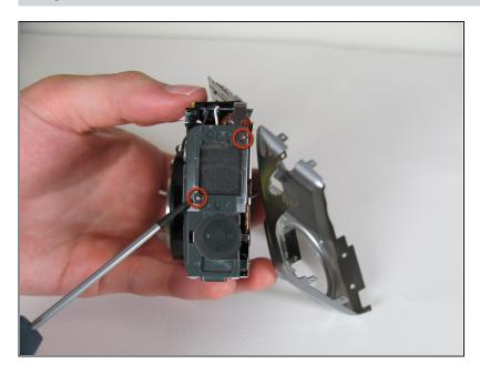
• Remove the two 2.9 mm screws on the right side of the camera.
