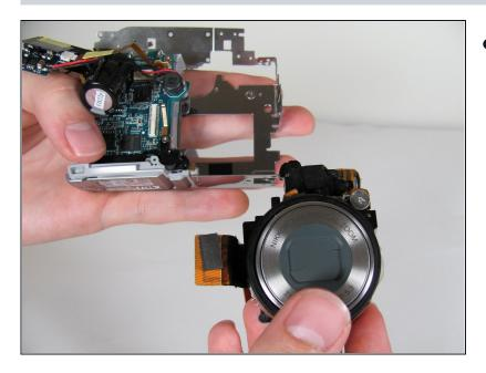
• Remove the lens from the rest of the camera.
