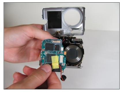
• Fully remove the motherboard from the camera body.
