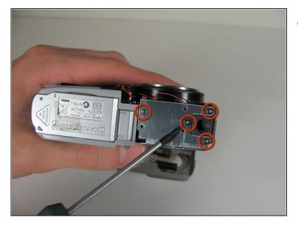
• Remove the four screws on the bottom of the camera.
