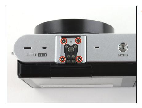
Remove the four 5 mm Phillips screws from the external flash mount.
