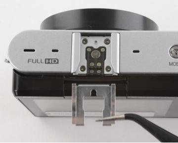
• Use tweezers to remove the metal shield from the external flash mount.
