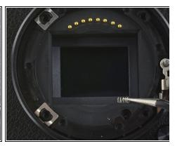
• Use tweezers to lift the pyramid screw and spring from the lens assembly.
