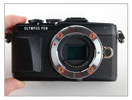
Use a Phillips #00 screwdriver to remove the four 6.3 mm screws from the lens mount.
