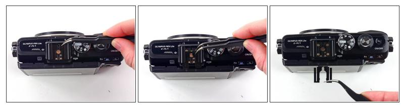
• Use tweezers to remove the metal clip from the external flash mount.
