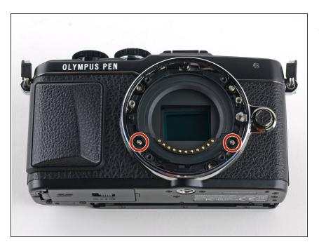
Remove the two 4 mm Phillips screws.
