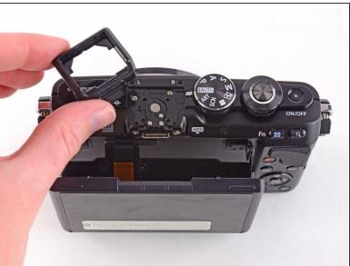
Remove the external flash port casing to expose five more screws.
