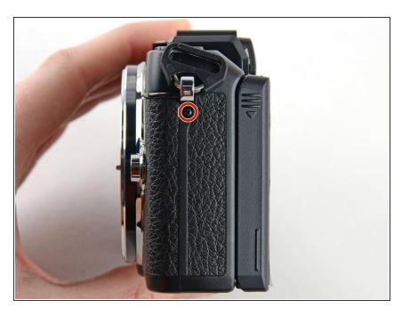
Use a Phillips #00 screwdriver to remove the 5 mm screw near the left hand grip.
