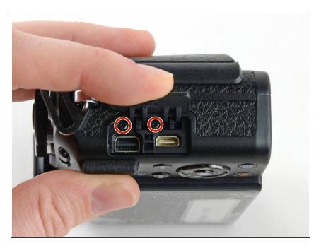
Remove the two 4 mm Phillips screws under the HDMI port cover.
