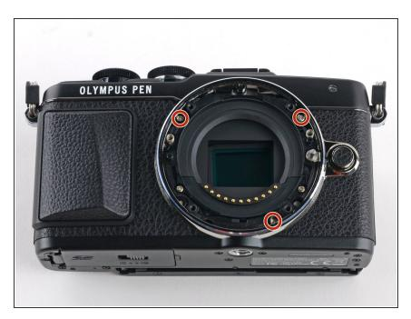
Use a Phillips #00 screwdriver to remove the three 5 mm screws.
