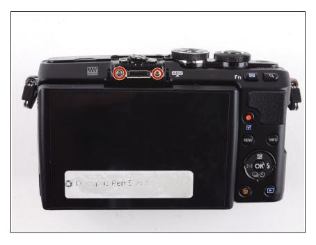
Remove the two 3.8 mm Phillips screws from the sides of the external flash connector.
