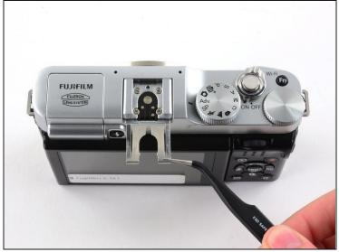
• Use tweezers to slide the metal shield straight out of the external flash mount.
