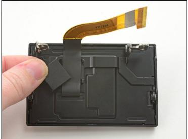
• Use the pointed end of a spudger to remove the ribbon cover on the back of the LCD.
