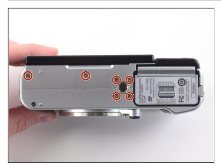
Remove the six 2.5 mm Phillips screws from the bottom of the camera.
