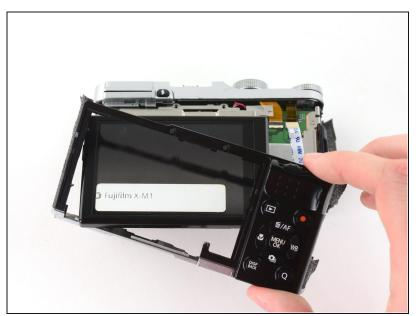
• Slide the frame around the LCD to remove it from the camera.
