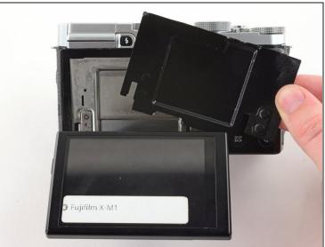
• Use two fingers to peel back and remove the black plastic cover from behind the LCD.
