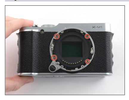
• Remove the four 4.3 mm Phillips screws inside the lens assembly.
