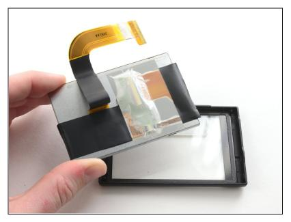
• Remove the LCD from the screen cover.
