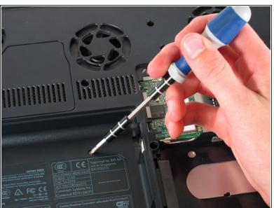
With the laptop face-down, remove the eleven 8mm Philips screws.
