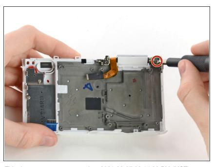
Remove the 5 mm Phillips #00 screw in the top right corner of the LCD assembly.
