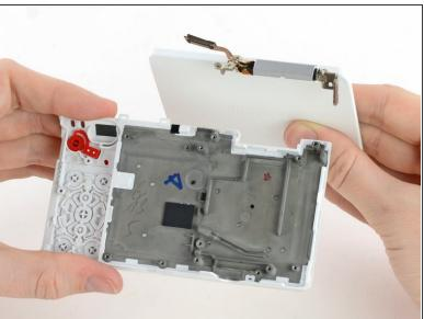
Tilt and wiggle the LCD to remove it from the case.
