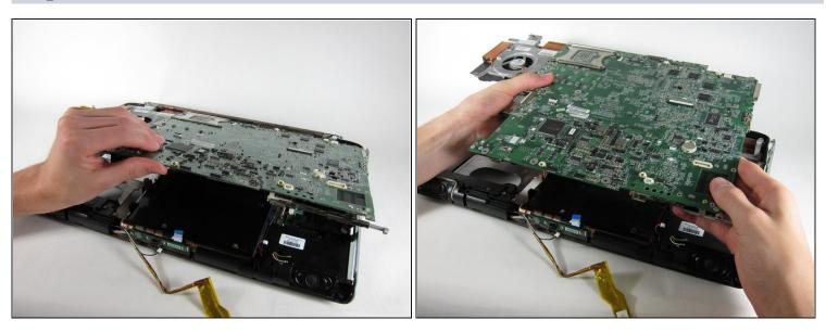
• Lift the motherboard up until it releases from the bottom casing and remove it from the laptop.
