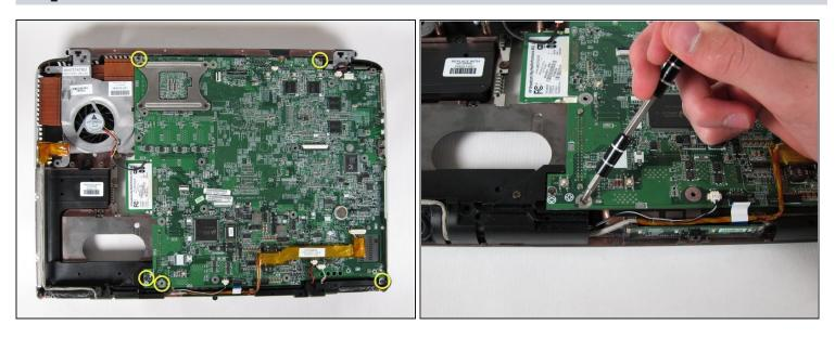
• Unscrew and remove the five 4mm Philips screws marked with the white Phillips screw icon.
