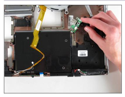
• Move the USB board out of the way and raise the right speaker unit up two inches.
