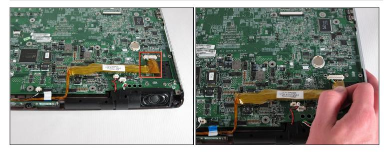
• Remove the audio cable - the one with the yellow covering located at the bottom-right corner of the motherboard - by pulling the yellow covering towards you.
