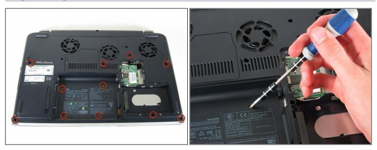
• With the laptop face-down, remove the eleven 8mm Philips screws.
