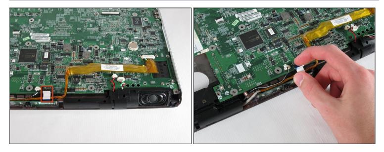
• Remove the LED board cable by pulling the white tab towards you.
