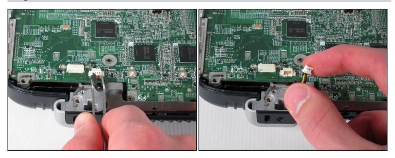
• Remove the fan cable by pulling the white connector away from you.
