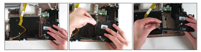
• Pull out the black cable running along the left side of the right speaker unit to remove it.
