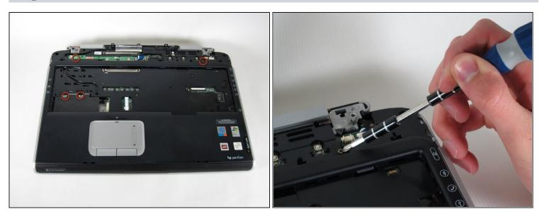
• Unscrew the four 8mm Philips screws from the top cover.
