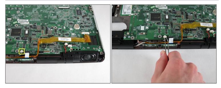
• Using tweezers, remove the left speaker cable by pulling the white connector towards you.
