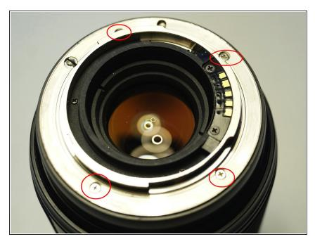
put the remaining parts back. Always tighten the screws very loosly at first and continue tighten them in a starway fashion (opposite sides).
