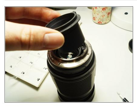
gently take aout the inner tube. Take care about the contact plate: it is connected with some fine wires to the optical parts and cannot be removed
