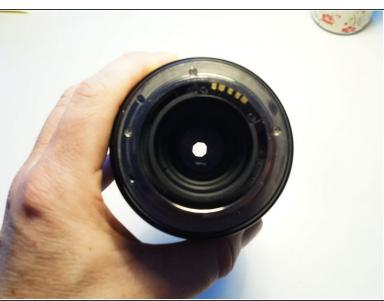
Move the lever back and forth and look through the lens: the aperture on a good lens should open and close and spring back into position
