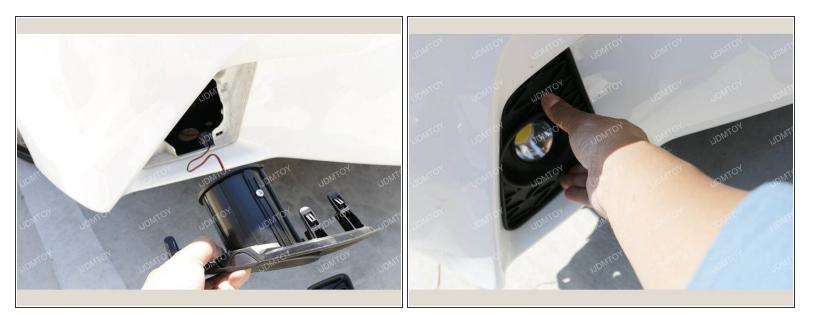
Insert your new Lexus GS F-Sport JDM Fog Lamps in the opening, starting with the wiring portion first. Then push in the Lexus GS F Sport Fog Lights into the lower bumper location. You will clear a loud CLICK once the tabs of your LED fog lamps lock in place.
