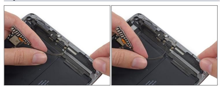
• Pull the antenna cable from the clip behind the Lightning connector.
