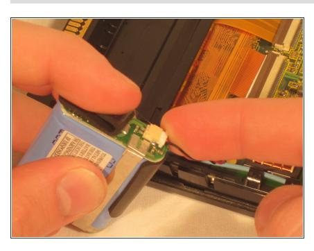
Attach the new battery by connecting it to the motherboard via the red wire.
