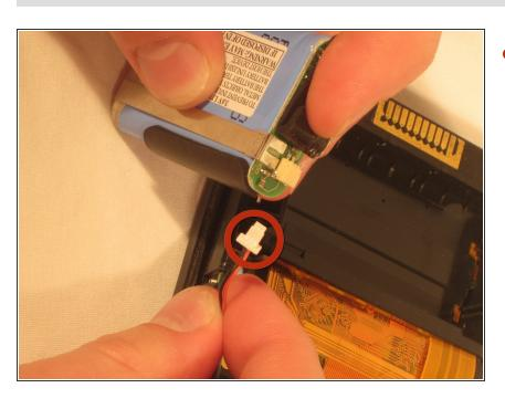
Detach the wire connecting the battery to the motherboard.
