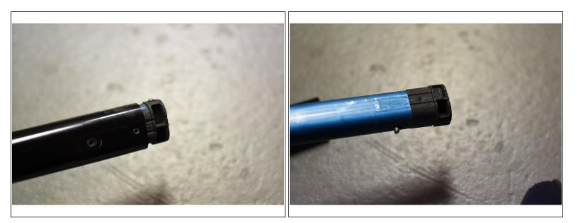
• Keep pushing the inner shafts down and push them so they come out the bottom of the outer shaft
