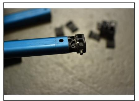
Press the innermost shaft through the bottom of the middle shaft and remove the bottom cap from that.
