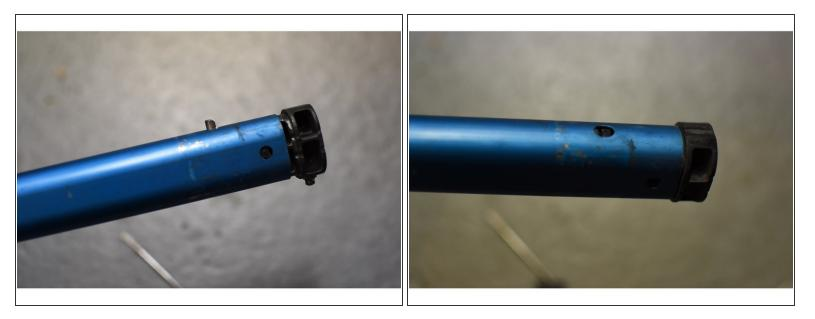
If you were able to get the inner shaft past the upper bushing, at some point the spring loaded pin popped out through the hole in the middle shaft. Press on the pin and push the inner shaft in a bit farther, then you can put on the other cap and bushings.
