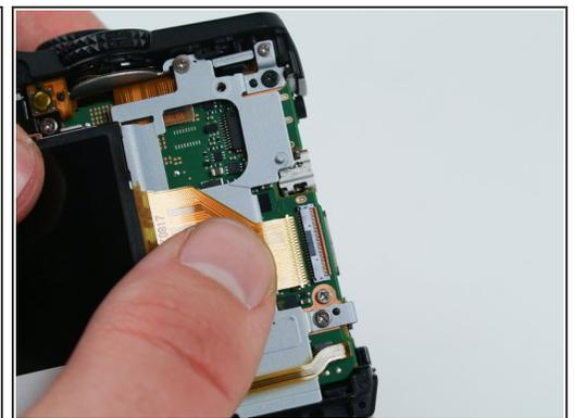
**⚠** Do not pull the connector upwards as doing so may harm the connector housing.
