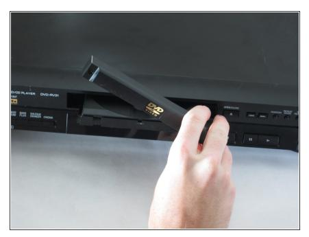
Evenly lift upward on the disk tray front cover (not slanted, as pictured). This will allow for easier disassembly of the player.
