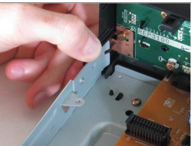
• Lift up the five tabs securing the front panel to the chassis. There are three on the bottom, and two on the inside edges of the panel. Panel should then lift off the player.
