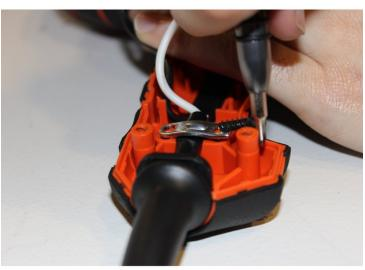
Using the T-handle screwdriver with the JIS 1 bit, unscrew the two lower black 12mm screws.
