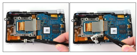
• Use tweezers to pull the tripod mount out of the front case.
