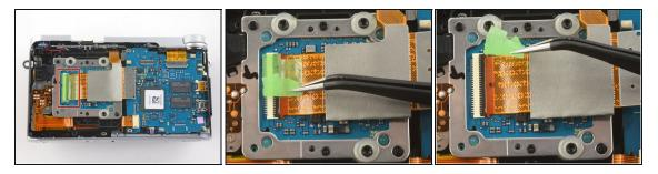
Use tweezers to remove the green tape covering the ribbon cable on the image sensor.
