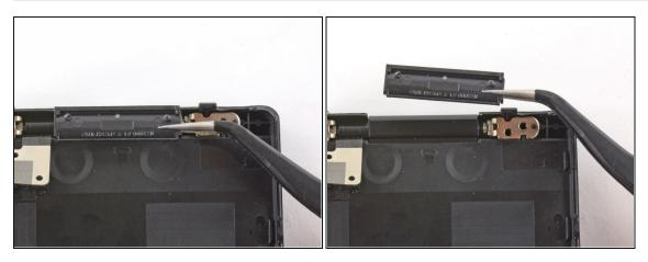
• Use tweezers to remove the plastic cover on the LCD hinge.
