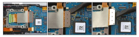
• Use the flat end of a spudger to disconnect the large ribbon cable by prying its metal connector straight up from the motherboard.
