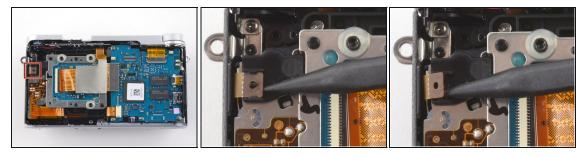
• Use the pointed end of a spudger to lift the ribbon cable straight out of the black clip located near the left handgrip.
