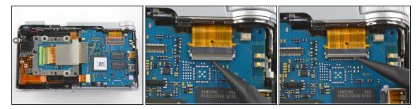
• Use the pointed tip of a spudger to unlock the ZIF connector by flipping the black bar straight up from the motherboard.
