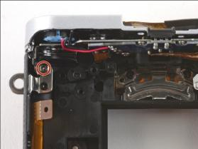
• Remove the 4.3 mm Phillips screw in the upper left corner that secures the top plate to the front case
