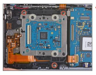
Remove the three 5.3 mm Phillips screws holding the sensor assembly in place.
