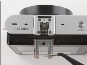
• Use tweezers to pull the metal shield straight out of the external flash mount.
