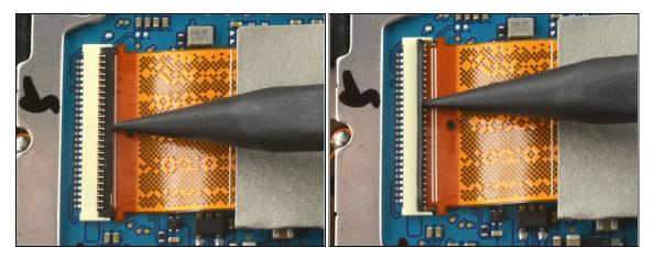
• Use the pointed tip of a spudger to flip the black bar on the ZIF connector straight up from the ribbon cable.
