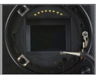
• Use tweezers to remove the pin and small spring from the lens assembly.
