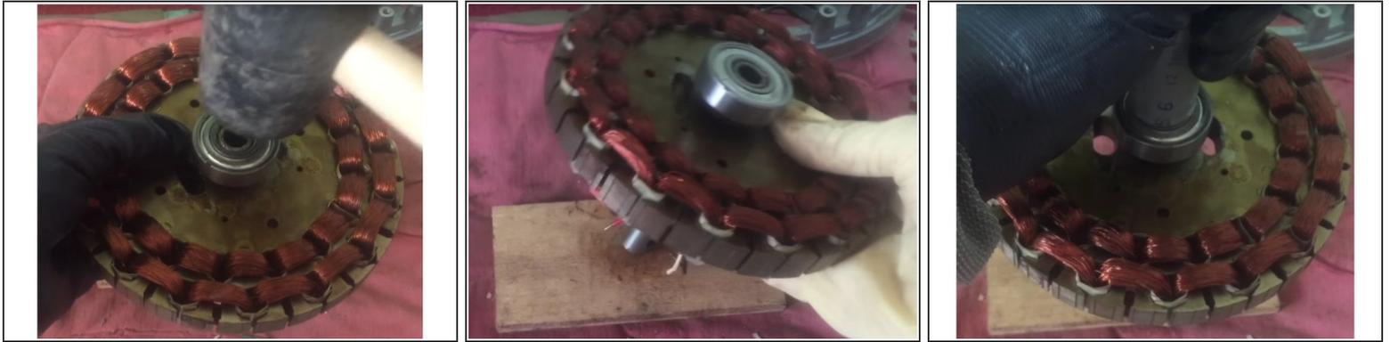
**⚠** Use a rubber mallet to install the other bearing onto the shaft. Rubber mallet or wooden mallet prevents damage to the bearing.
