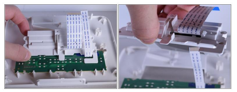
• Carefully remove the frame attached to the screen.
