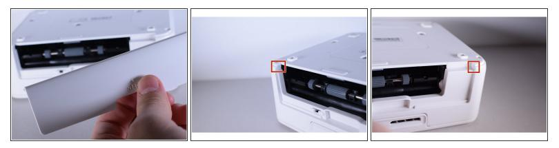
• Turn the device around and remove the "open" lid.
