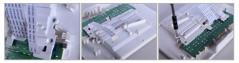
Use the PH0 screw bit to remove the five 10 mm screws located above the circuit board.
