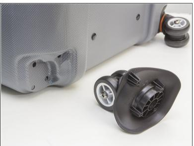
Remove the wheels from the wheelhouse.
