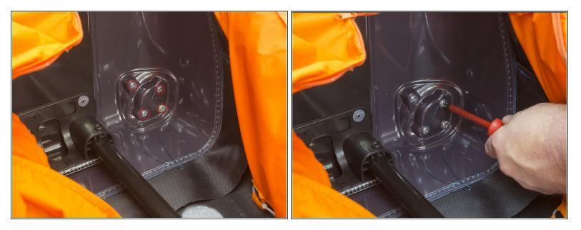
Unscrew the 4 screws with a Phillips screwdriver PH2 die 4.
