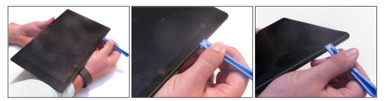
$\triangle$  Avoid prying near bottom right hand side due to LCD Connector
