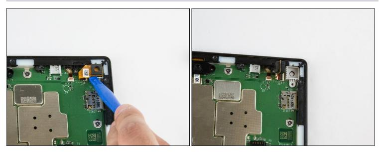
• Lift the camera from the case using the plastic opening tool.
