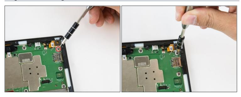
• Remove the single T5 Torx screw at the base of the camera.
