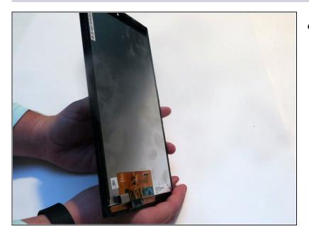
Remove the screen and digitizer from the case completely.
