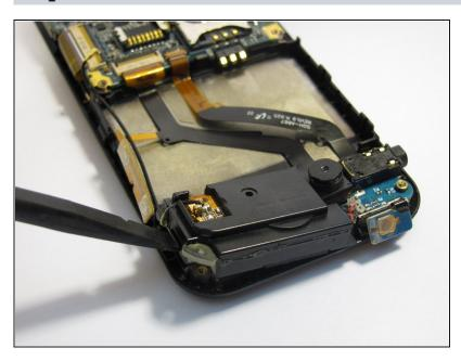
Pry the antennae/speaker component out of its casing. You need to use a little force to get the piece to pop out.
