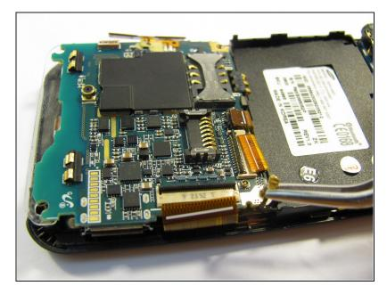
Pop the antenna plug off of its socket with a pair of metal <u>tweezers</u>.
