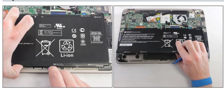
Gently lift up the battery and remove using the plastic opening tools.
