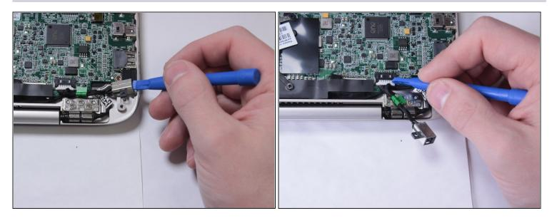
• Lift out and disconnect the charge port.
