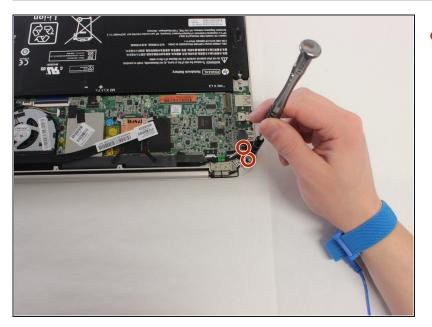
• Remove the two 2.0 mm screws in the charge port bracket using the PH00 screw head.
