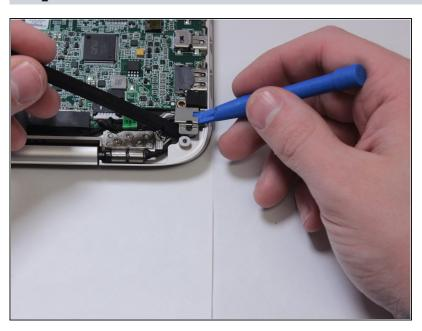
Use the plastic opening tools to remove the bracket.
