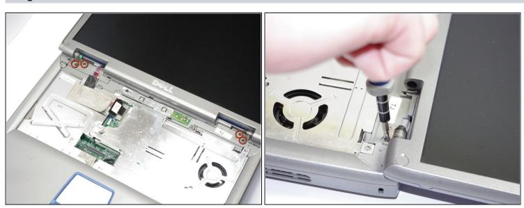
• Using a Phillips screwdriver remove the four screws (5.8 mm) located at hinges of the screen.
