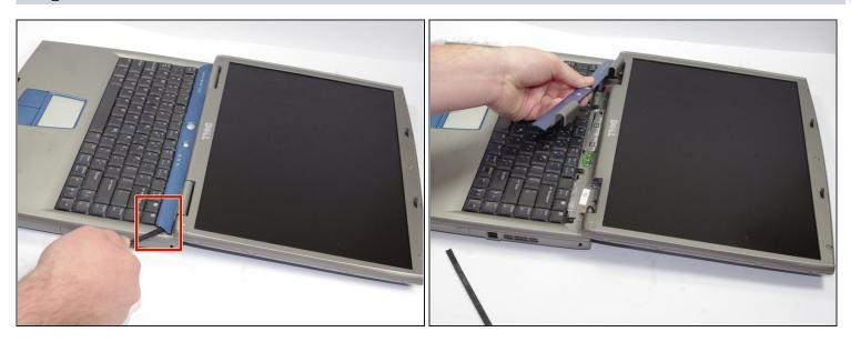
• Starting from the right side of the hinge cover, use the flat end of the spudger to pry up the hinge cover and gently remove it.
